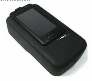
The *Handheld Raman* packs a-full featured Raman Spectrometer system in a remarkably affordable true handheld format. The lightweight unit is controlled by a pocket-size Windows® computer and features easy-to-use software that provides one-touch identification of unknown substances by immediate comparison of a measured spectrum to the on-board Raman spectral library.
